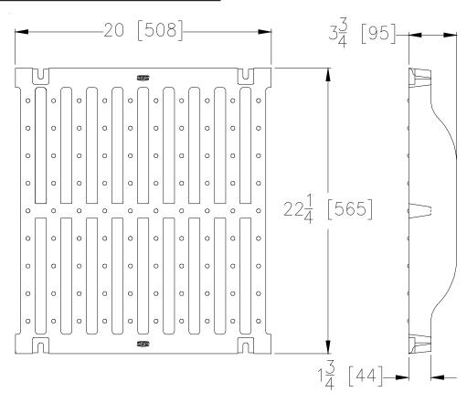
**ENGINEERING SPECIFICATION:** The Zurn -DGF, Ductile Iron Slotted Grate, is 22-1/4" wide x 20" long, weighing 73.4 lbs per linear foot. The grate has an open area of 94.1 square inches per linear foot, DIN Rating of Class F, ANSI Rating of Special-Duty, H-20 Load Rated and FAA Load Rated.
